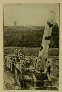
Camouflaged Big Gun. Mounted on a specially constructed railroad carriage, this big French 400 m/m, gun was ready to bang away at the German forces making the drive on the Somme front. It was exceedingly well camouflaged to prevent detection by Boche aerial forces.
